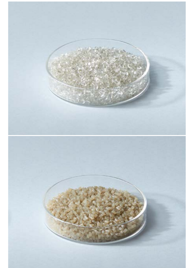
OBP PET and OBP PA pellets made from marine waste PET bottles and fishing nets
